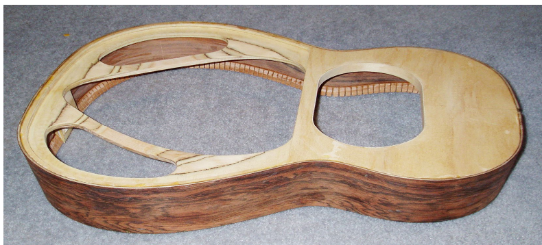
Fig. 3: Guitar carcass, showing laminated skeleton reinforcement for the sides.
